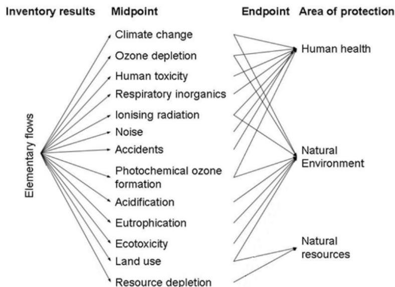
Figure 13: Framework of impact categories for characterization modeling at midpoint and endpoint levels
