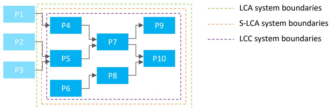
Figure 6: Identical system boundaries, case a: practical approach
