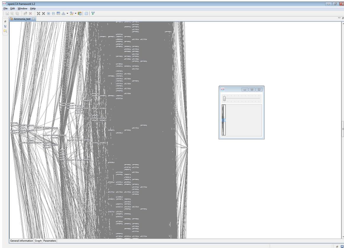
**Figure 3: Example for a graphical display of a product life cycle (ecoinvent 2.2 database, ammonia production, displayed in the openLCA software; one box represents one process)**
