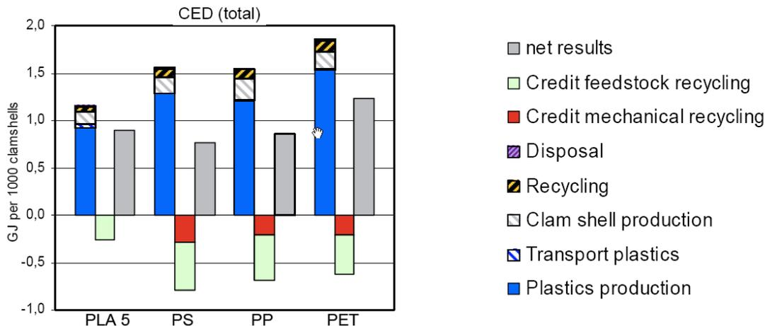
Figure 5: Cumulative energy demand as result of an (environmental) LCA study with negative demand for some parts of the life cycle due to system expansion (avoided product) calculations
