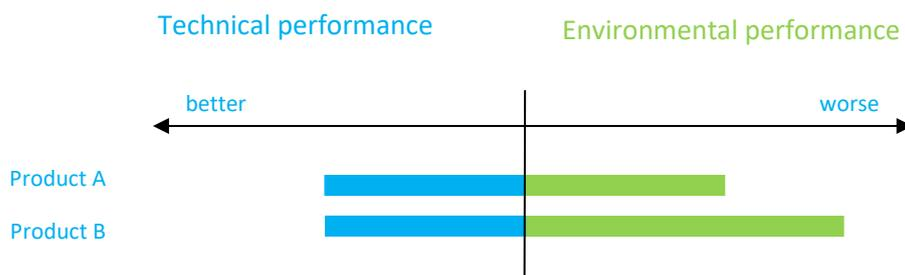
Figure 4: The principle of a functional unit in LCA: with identical technical performance, the environmental performance of products can be reasonably compared in order to identify the best alternative (here: product A)
